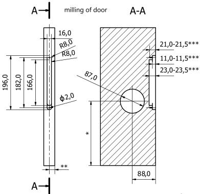
\* according to the door manufacturer's custom \*\* fitting / positioning of the Magnetic block in the door must be solved following the seating of the Magnetic in the doorframe \*\*\* placing of the magnetic block face according to the door manufacturer's custom
